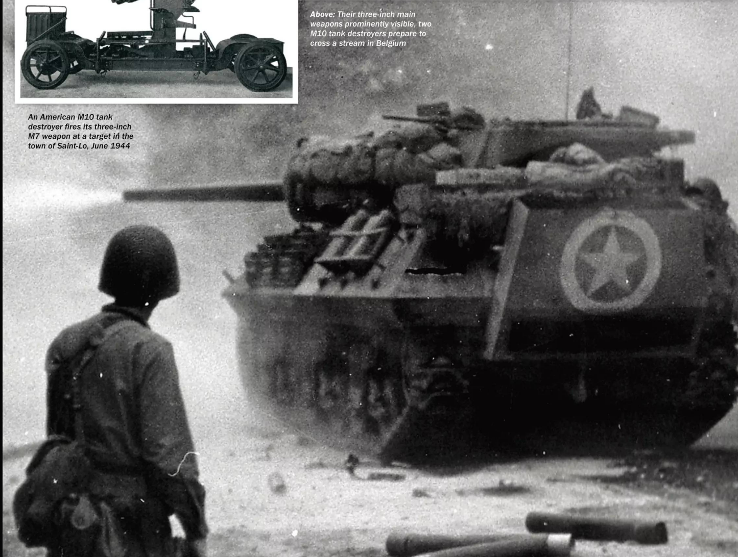
The three-inch Gun M1918 anti-aircraft weapon was modified as the M7 for use in the M10 and M10A1 tank destroyers
